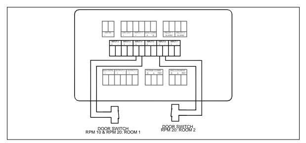
Figure 26. Optional Door Switch Wiring to Model RPM10/RPM20
