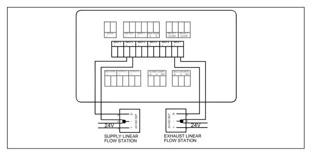
Figure 24. Optional Supply/Exhaust Linear Flow Station Wiring to Model RPM10/RPM20
