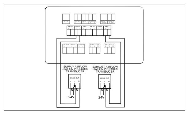
Figure 23. Optional Supply/Exhaust Pressure-Based Flow Station Wiring to Model RPM10/RPM20
