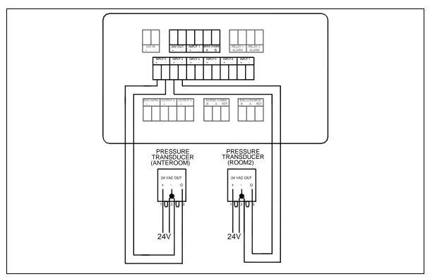
Figure 21. Optional Room 2 and Anteroom Pressure Transducer Sensor Wiring to Model RPM20
