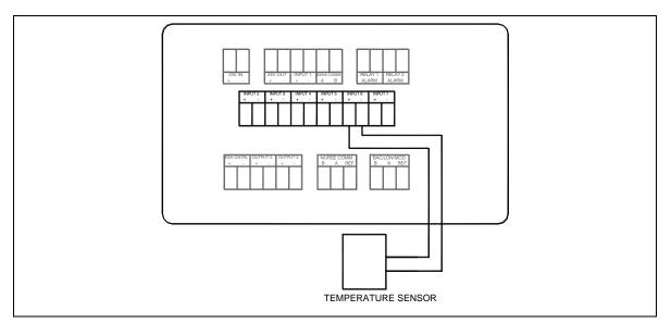
Figure 28. Optional Temperature Sensor Wiring to Model RPM20
