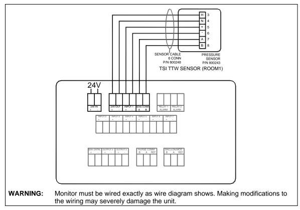
Figure 18: Wiring Diagram – Through-The-Wall Sensor Wiring to Model RPM10/RPM20
