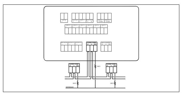
Figure 32. Optional Nurses Station Communications Wiring to Model RPM10/RPM20
