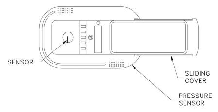
Figure 13: Pressure sensor door slid open
