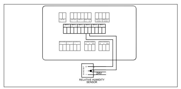
Figure 31. Optional Relative Humidity Sensor Wiring to Model RPM20
