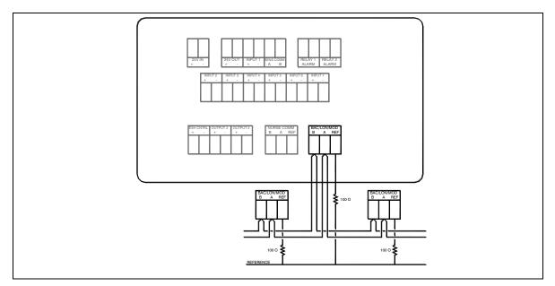
Figure 33. Optional Modbus and BACnet MS/TP Communications Wiring to Model RPM10/RPM20
