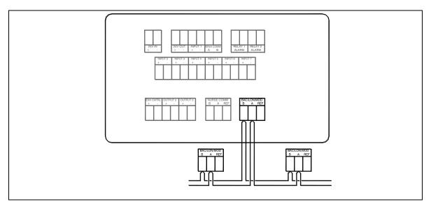
Figure 34. Optional LONworks Communications Wiring to Model RPM20-LON
