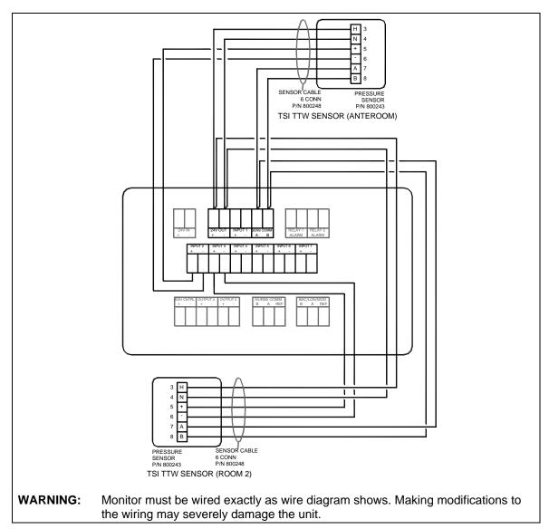
Figure 19: Optional Room 2 and Anteroom Through-The-Wall Sensor Wiring to Model RPM20
