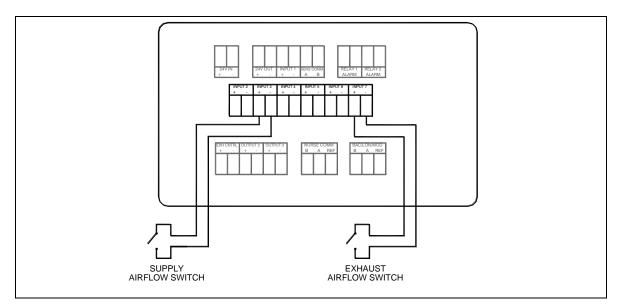
Figure 22. Optional Supply / Exhaust Flow Switch Wiring to Model RPM10/RPM20
